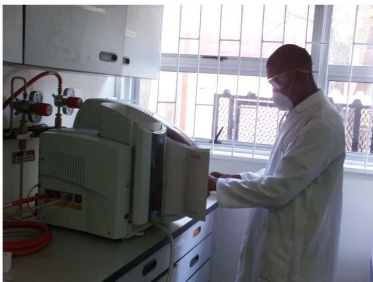
Plate 2: Inserting correct lamp in the AA machine
